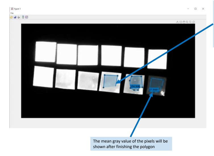
Left click to enter a new vertex. After closing a polygon with the last vertex, right click into the polygon area and select "finish" from the menu to finish polygon. Note, that this process will repeat several times according to the number of AOIs selected in the calibration menu. You are able to delete a single vertex, however do not delete the last one. If so, you need to close the window and start AOI selection again
